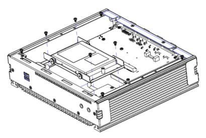
Step3. Please loosen 4 screws to remove the HDD bracket from board & system assembly.
