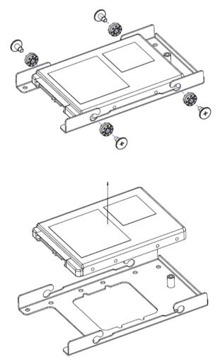
Step 4.1 Remove 4 screws to release the HDD bracket.
